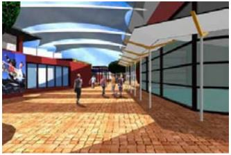
Fabric tensile structure  $oldsymbol{\underline{1}}$
